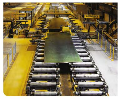
Following the joining process, the plates are manipulated on a plate bending machine capable of facilitating very large diameters. With a roller table for fast loading, side support manipulators and precision laser checking for roundness tolerances, the Haeusler bending machines are available in a variety of options to suit the demands of the customer.
